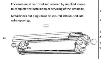
Wiring may be terminated within the enclosure, or may terminate at the junction box remote from the luminaire.
