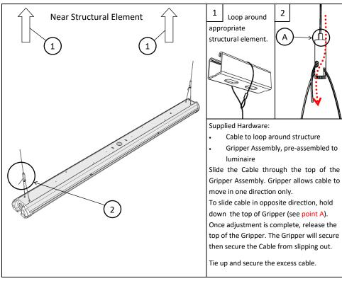
Part of the suspension kit is assembled into the light fixture. However, if for some reason the suspension kit is not completely assembled into the fixture, follow the following procedure to reattach the cable into the luminaire.
